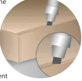
the sponge from drying out. The applied hydrophobing agent should be allowed to soak in for 24 hours. After that, the treated surface can be exposed to moisture again.
